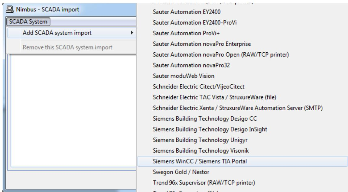
In *Nimbus Explorer* select *Setup -> SCADA import setup*. Select *SCADA System -> Add SCADA system import -> Siemens WinCC / Siemens TIA portal*
