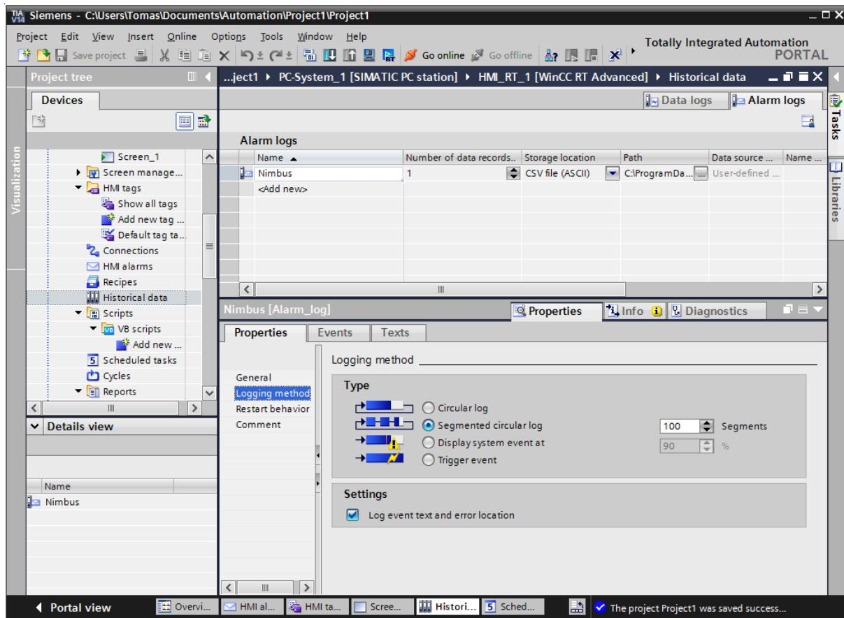
Select *Segmented circular log* and at least 100 segments - this actually means upto 100 simultaneously alarm events between Nimbus file scans which defaults to 2000 msec.
