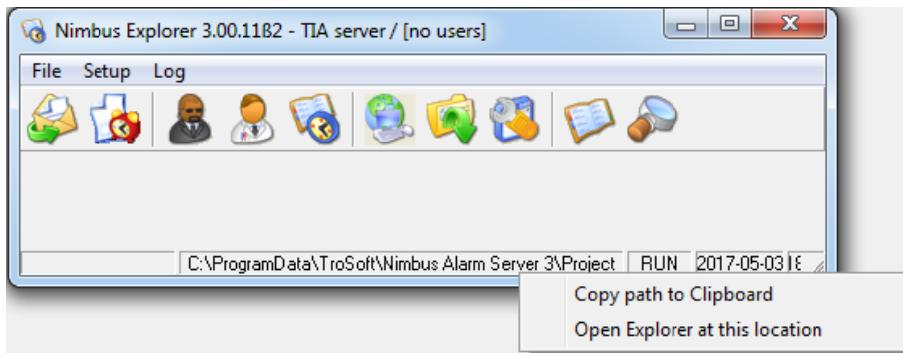
First of all create an *Alarmlog* folder where both TIA and Nimbus have *Full control (read/write/delete file access)*. A good place is where Nimbus data resides - you see the path down right in Nimbus Explorer.
