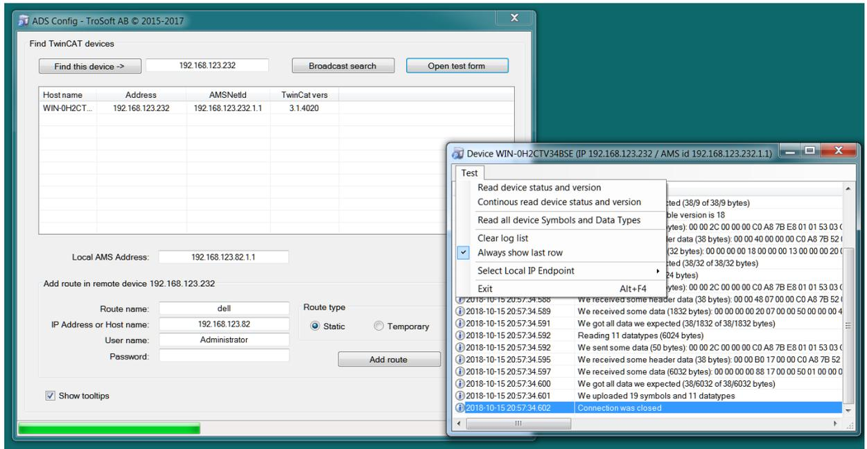
Sample of how the tool can be used to scan for devices on the local subnet using broadcast search and to test communication. In the above example the router line to the is ok and we get a proper response from the device.
