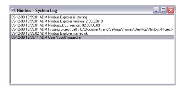
In the list date and time and originator is shown, i e *SRV* for *Nimbus Alarm Server* and *ADM* for *Nimbus Explorer*. The message itself is somewhat self explanatory and will not be further explained here.
