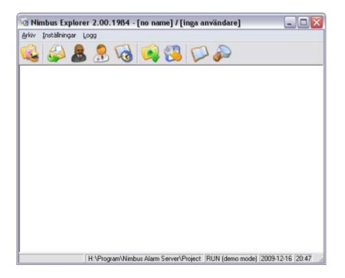
The window caption shows the program version, server name and any logged-in user. In the bottom information field the current status, projectfolder and if *Nimbus Alarm Server* is running or not (STOP/RUN/BLOCK), date and time is shown.
