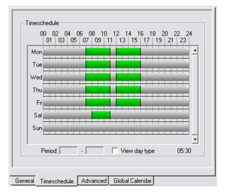
The timeschedule shows with green columns the times the profile is active. The interval is between 00:00-24:00 with a resolution of 5 minutes.
