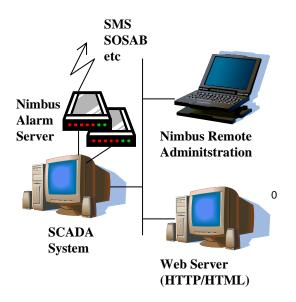
*Nimbus Alarm Server* is most frequently installed on the SCADA systems' alarm- or I/O server. *Nimbus Alarm Server* is administrated in the same server it is installed in or via the ActiveXobjects appended.
